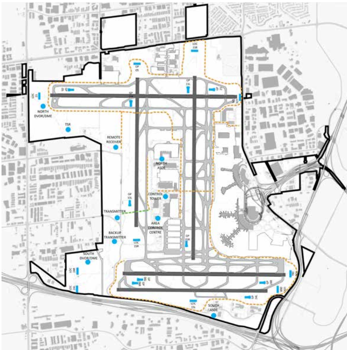
Figure 6-2: Existing ATC and CNS Facilities
