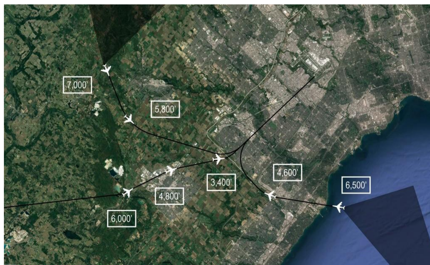
Left: Map shows the composite proposed approaches to Runway 06L in black; shaded areas show where there is expected to be some traffic distribution prior to joining the procedure. Aircraft icons show the approximate altitude on points along the procedure.
