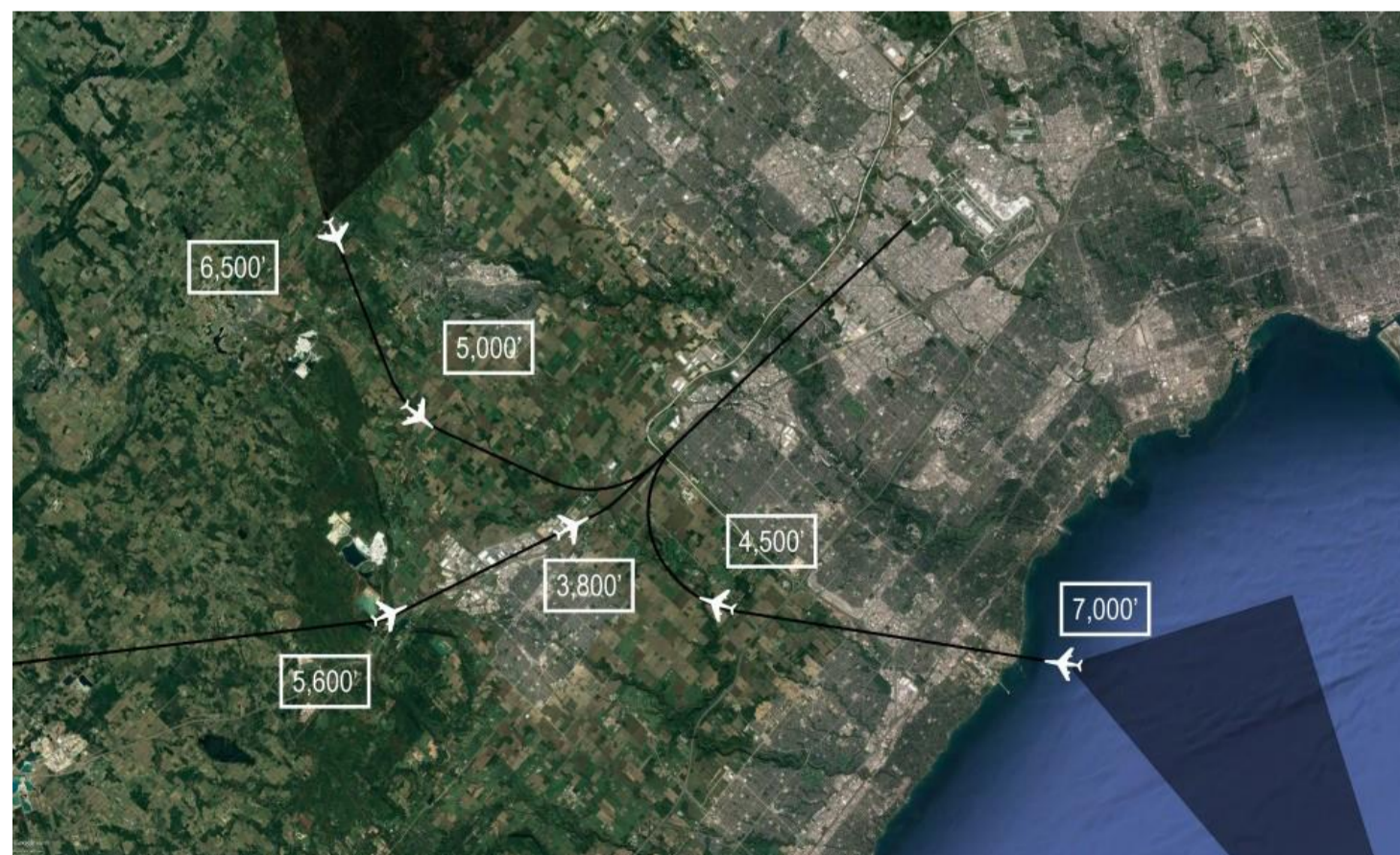
Left: Map shows composite proposed approaches to Runway 05 in black; shaded areas show where there is expected to be some traffic distribution prior to joining the procedure. Aircraft icons show the approximate altitude on points along the procedure.
