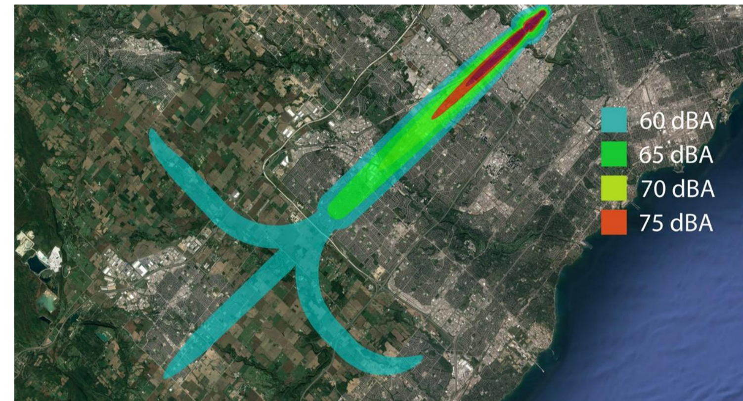
Above: Map shows the modeled noise footprint of an aircraft (737-800) flying the arrival procedure. Noise analysis suggests that as many as 27,000 fewer people will be affected by noise levels >60dBA from overnight flights when Runway 06L is in use. This represents a reduction by as much as 13 per cent depending on the approach.
