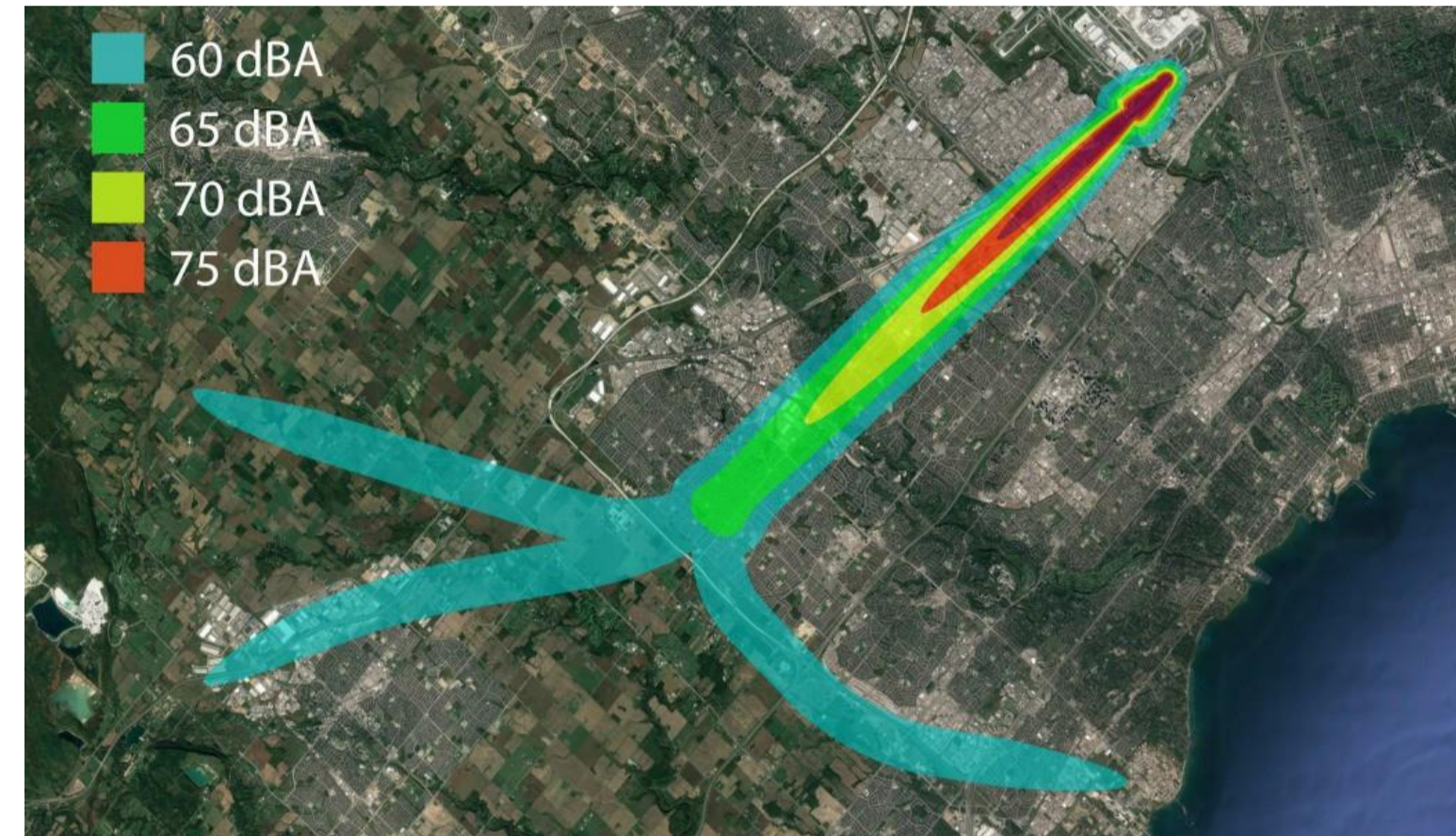
Above: Map shows the modeled noise footprint of an aircraft (737-800) flying the approaches. Noise analysis suggests that 34,000 fewer people will be affected by noise levels >60dBA from overnight flights when Runway 06R is in use. This represents a reduction by as much as 30 per cent depending on transition flown. It should be noted that 06R is not a nighttime preferential runway and usage of this runway at night will be low.
