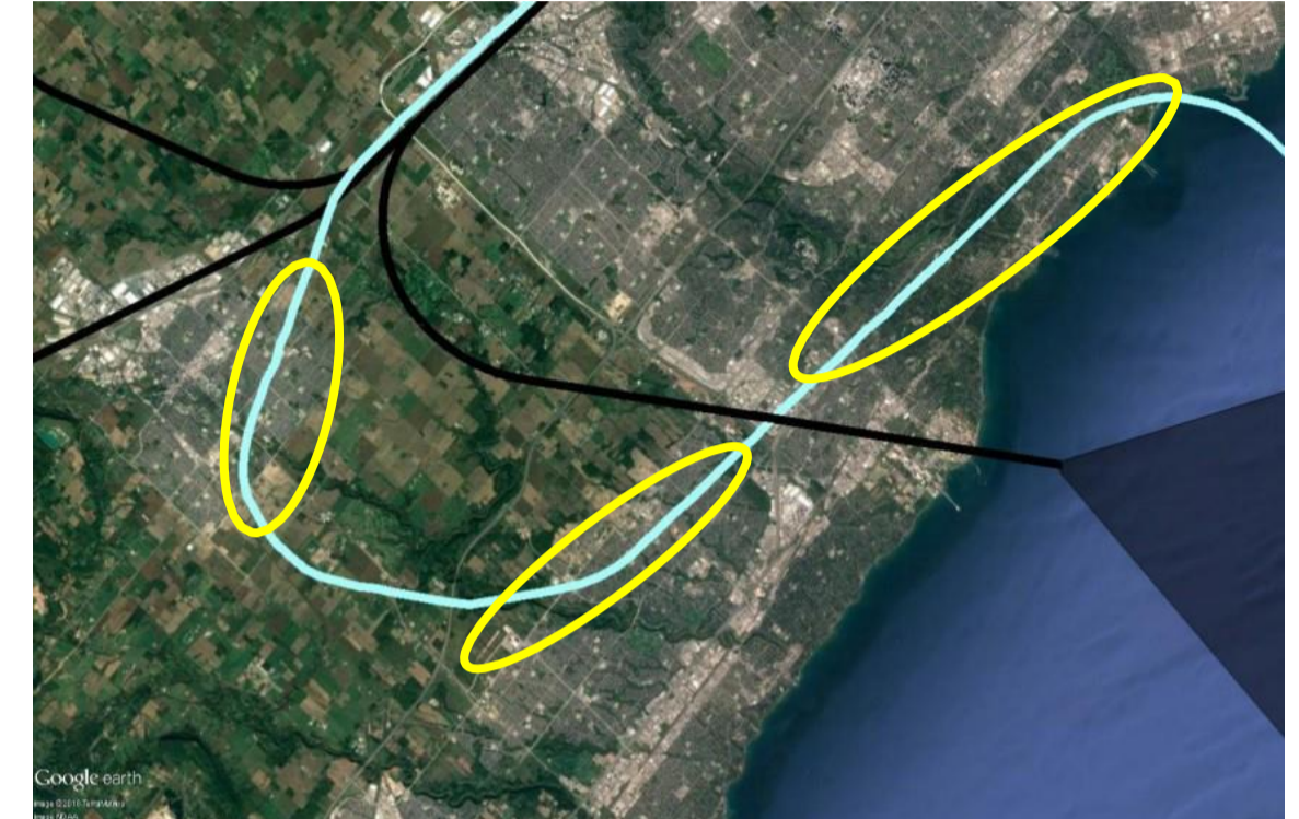
The light blue line below shows an example arrival using a downwind leg, with residential areas circled in yellow. These will be avoided when an aircraft employs the proposed approach (black).
