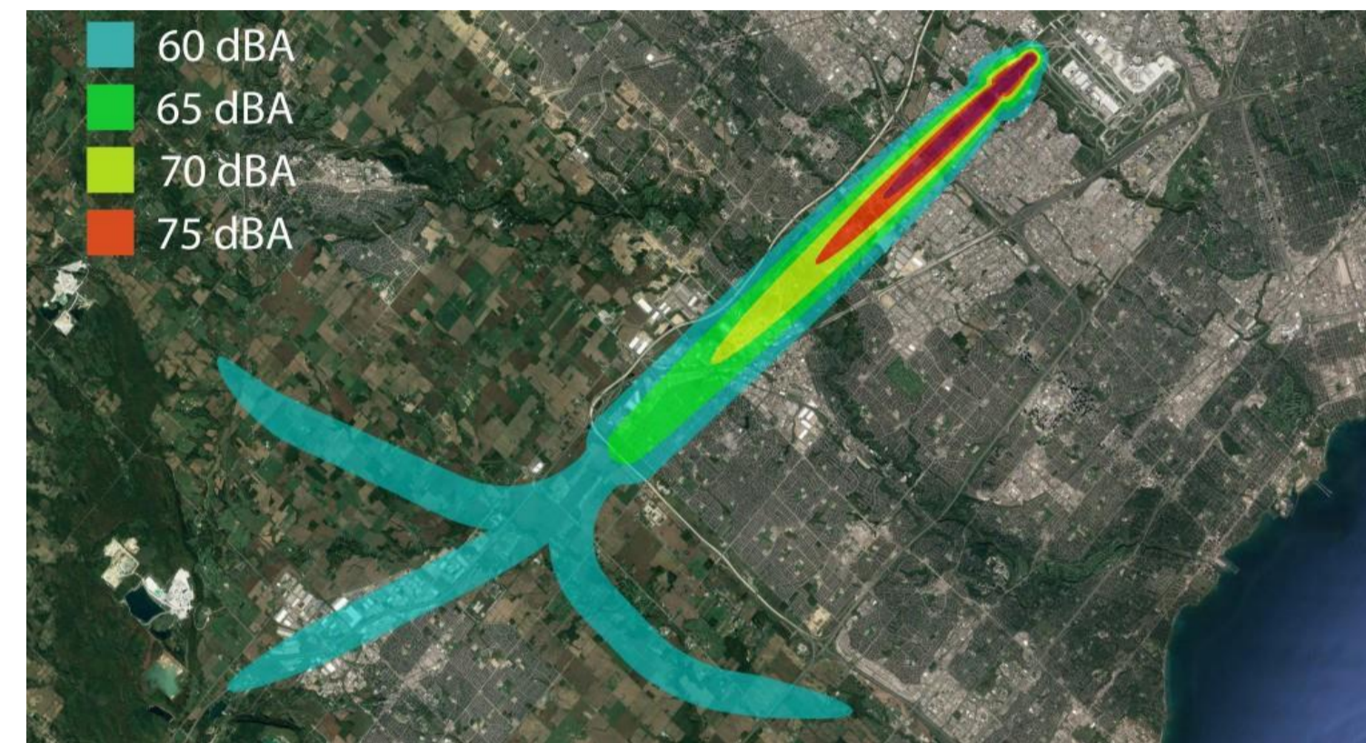
Above: Map shows the modeled noise footprint of an aircraft (737-800) flying the approaches. Noise analysis suggests that 29,000 fewer people will be affected by noise levels >60dBA from overnight flights when Runway 05 is in use. This represents a reduction by as much as 22 per cent depending on transition flown.
