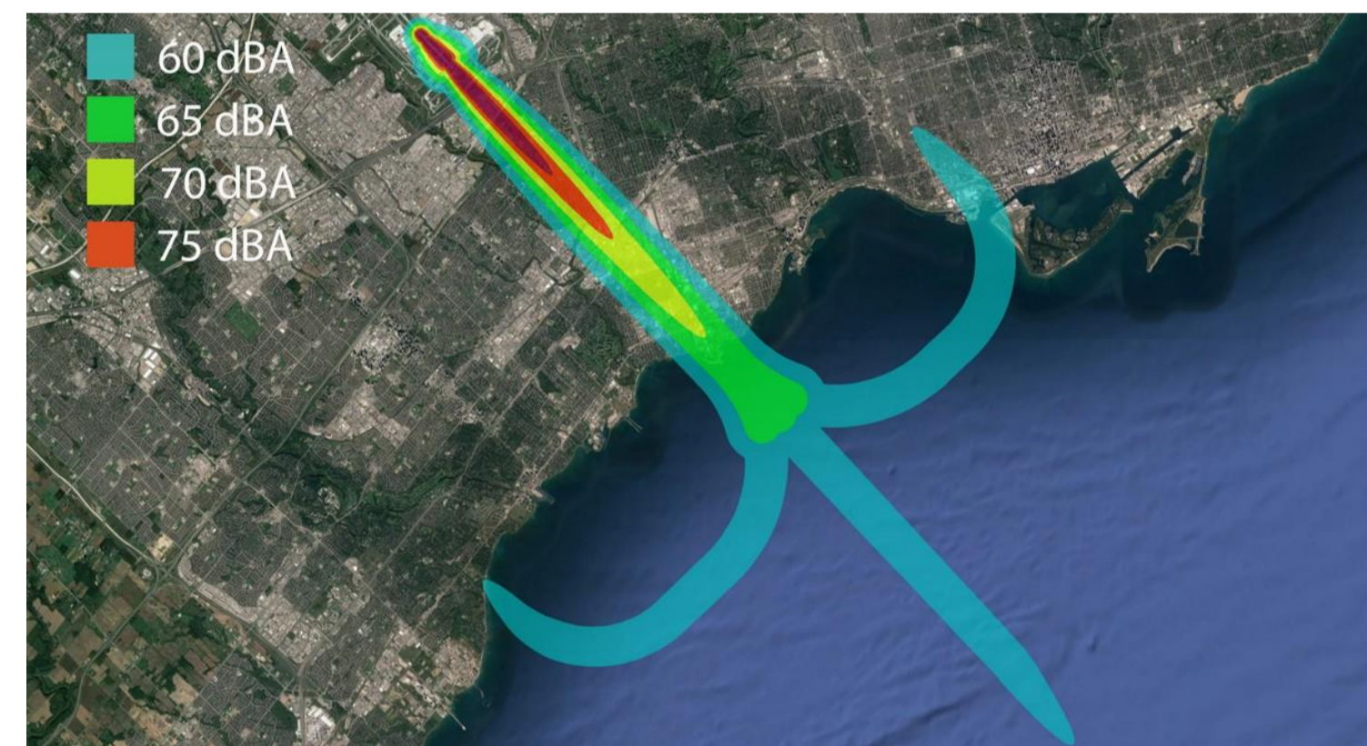
Above: Map shows the modeled noise footprint of an aircraft (737-800) flying the arrival procedure. Noise analysis suggests that as many as 27,000 fewer people will be affected by noise levels >60dBA from flights when Runway 33L is in use. This represents a reduction by as much as 24 per cent depending on the approach.
